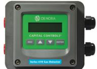
The optionally available auto-testing feature provides assurance that the detector is always ready should a leak occur. The generator test cell produces a small quantity of gas right below the sensor element to verify the sensitivity to gas. Testing can be scheduled to occur at a preset time every day or week with the results logged allowing for seamless automatic testing functionality.
